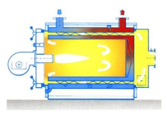
For this reason so called. ,,centrifugal type", efficiency-improving, spiral-flow retention elements were designed. As these turbulators are situated in the tubes' final stage, so reducing danger of acidic condensation.
